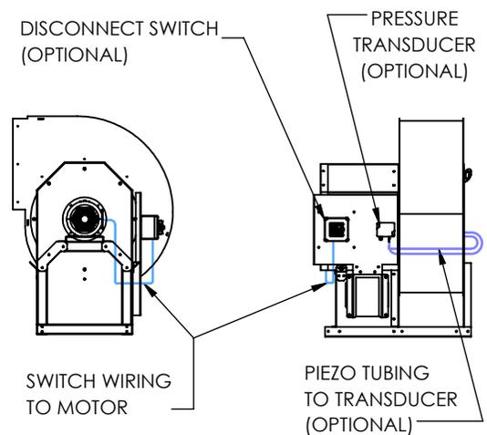
**ARRANGEMENT-4 WITHOUT ONBOARD SPEED CONTROLLER**
