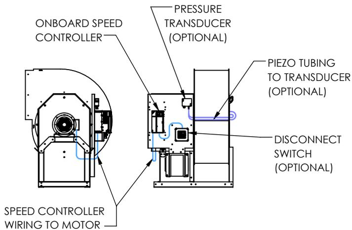
**ARRANGEMENT-4 WITH ONBOARD SPEED CONTROLLER**
