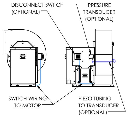
**ARRANGEMENT-10 WITHOUT ONBOARD SPEED CONTROLLER**
